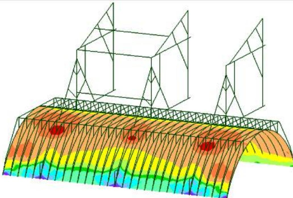
Inside-strain in the  $N_{xx}$  plate (kN/m) along the curve
