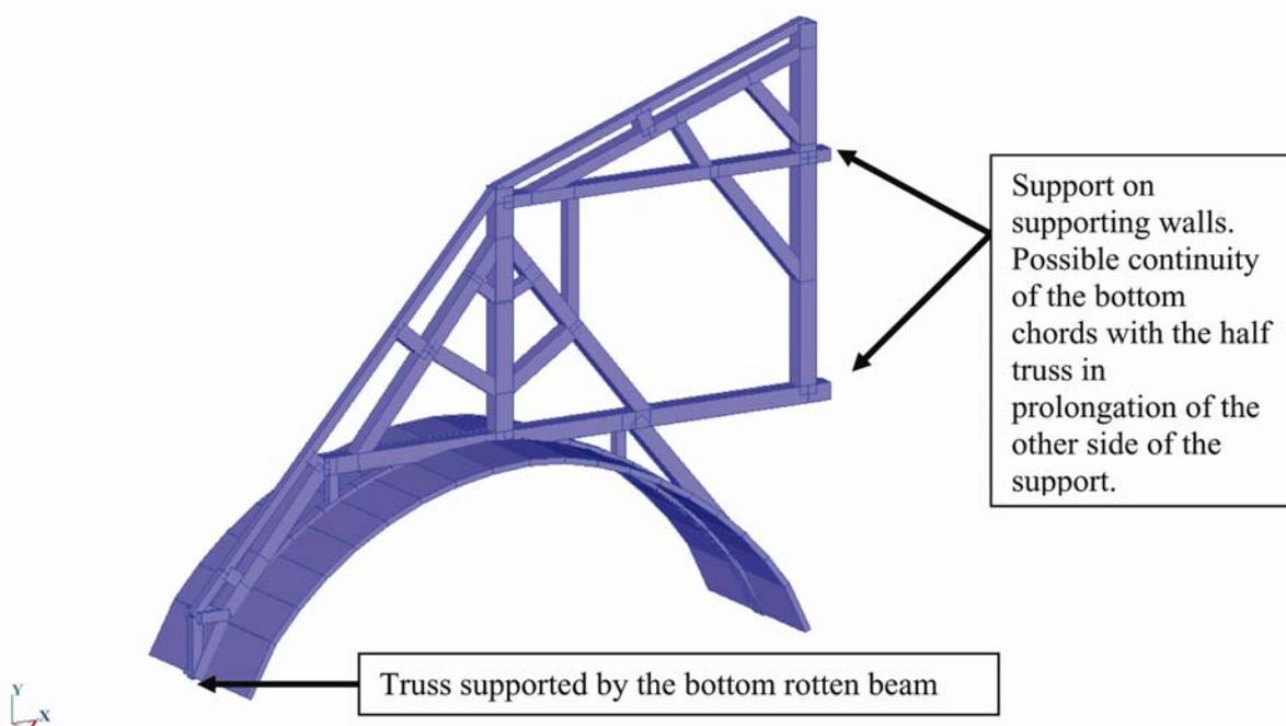
For each truss, the permanent roof loads are 3,3 kN/m, and the climatic loads are limited to snow, more unfavourable than wind, i.e.:
