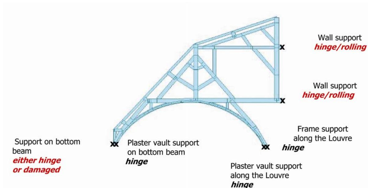
The unknown supports (bottom beam and wall supports) vary :
