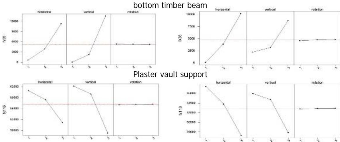
**➔ Load transfer from the bottom timber beam to the plaster vault**
