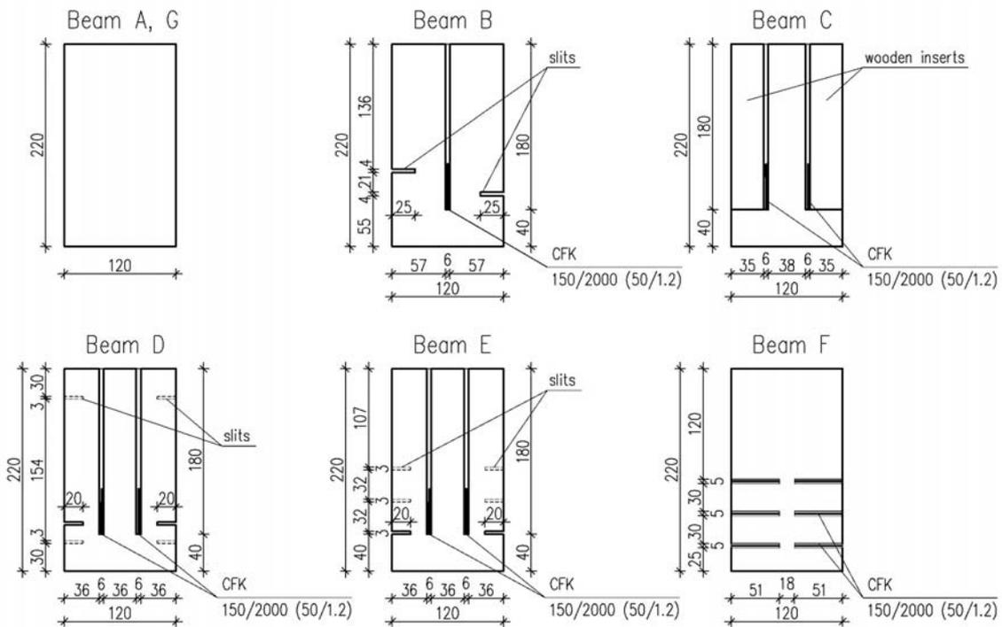
Figure 2. Cross sections of tested beams
