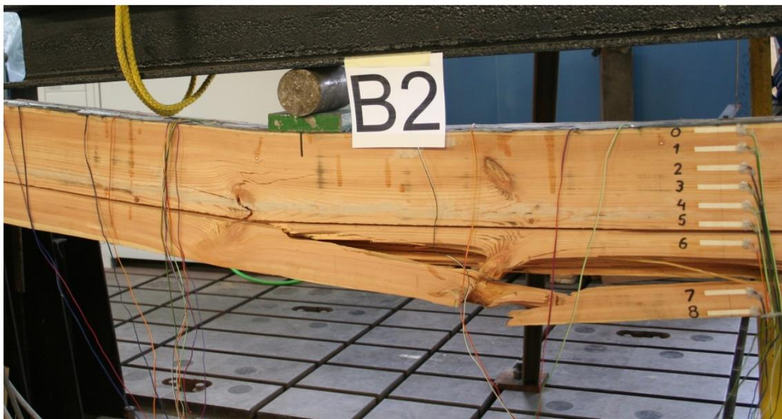
**Figure 9.** Form of destruction of beam B2
