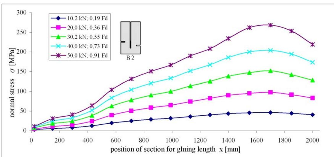
Figure 7. Normal stresses of strip - beam B2
