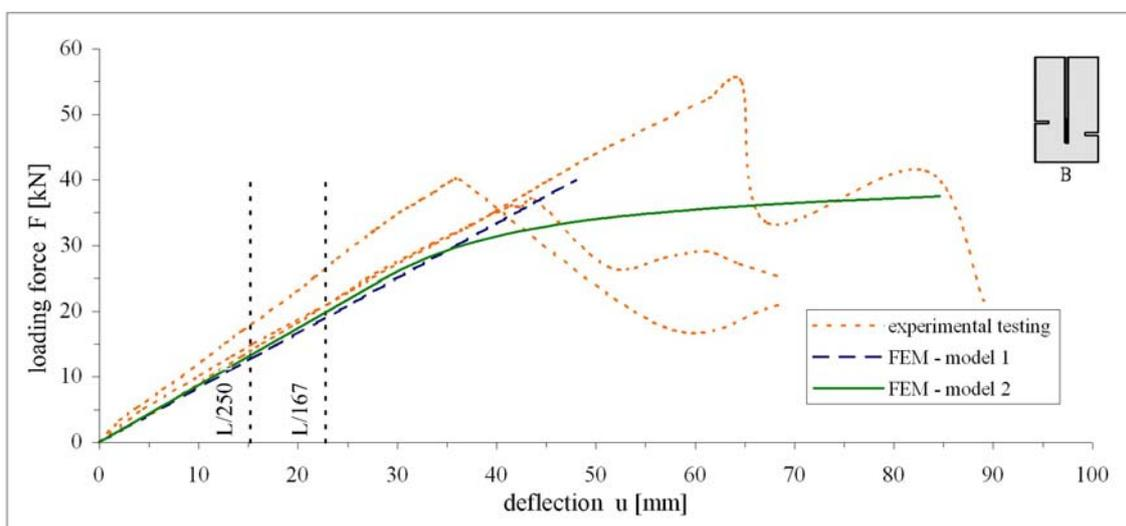
**Figure 13.** Relationship of "F" for experimental models and numerical testing, beam
