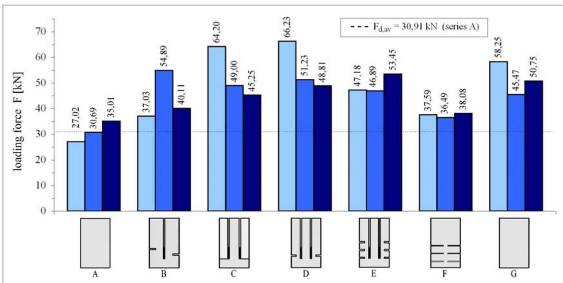
**Figure 4.** Values of destructive force of tested elements
