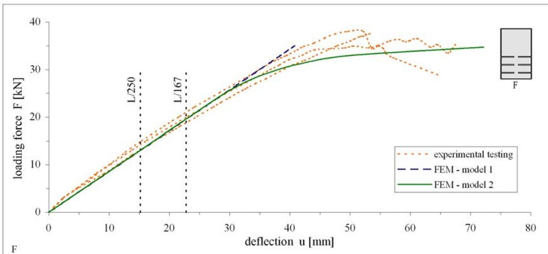
Figure 14. Relationship of "F" for experimental models and numerical testing, beam F
