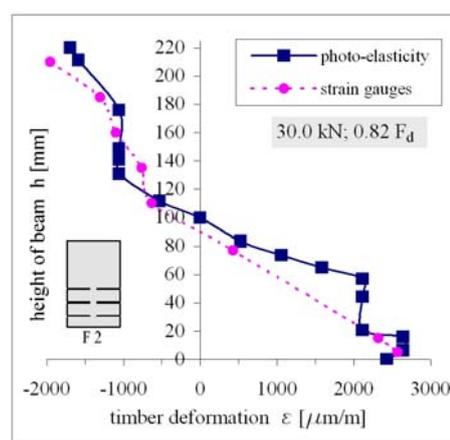
**Figure 12.** Timber deformation in bent section – beam F2
