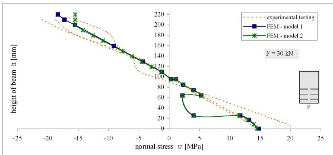
Figure 16. Graph of normal stresses in wood in beam F, force F = 30 kN
