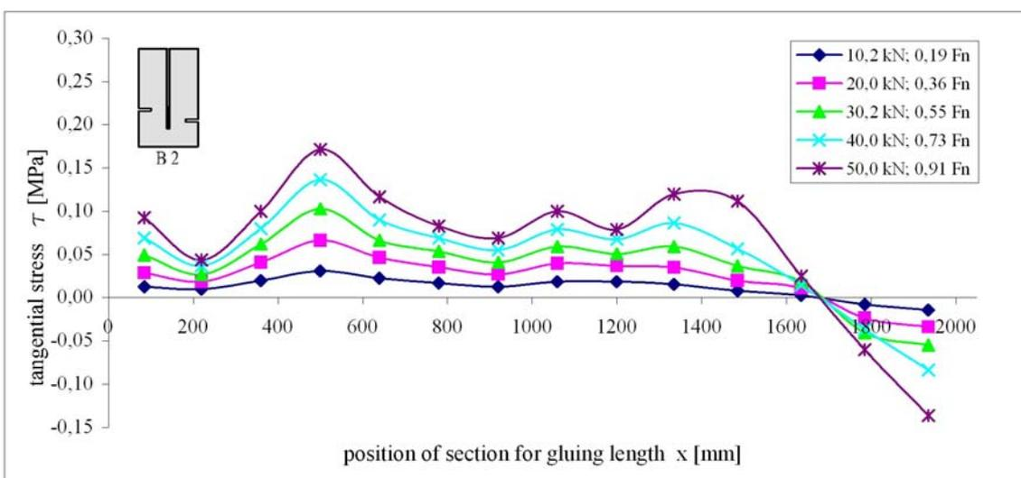
Figure 8. Tangential stress in joint - strip in beam B2
