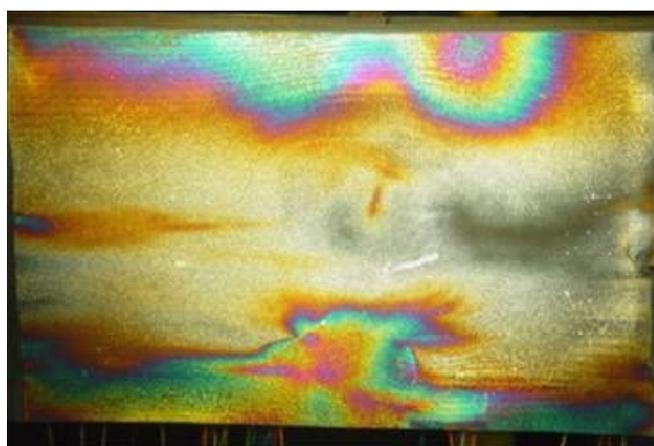
**Figure 11.** Total isochromatic image – beam F2
