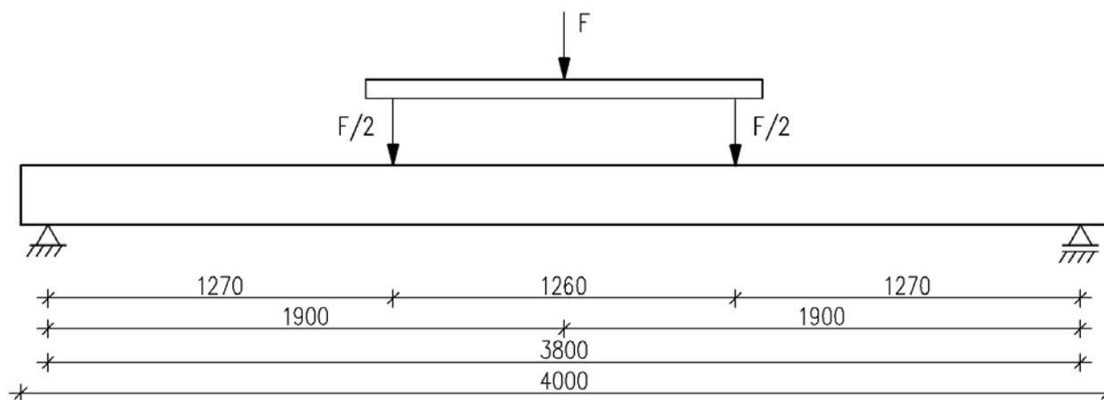
**Figure. 1** Testing station diagram
