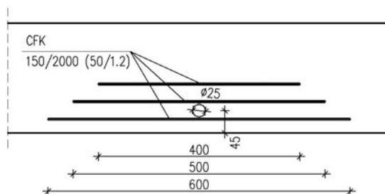
Figure 3. Maximum bending moment zone of beam F, side view
