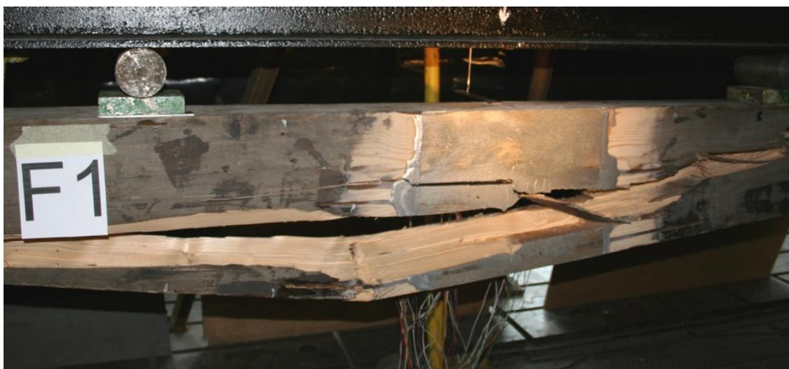
**Figure 10.** Form of destruction of beam F1
