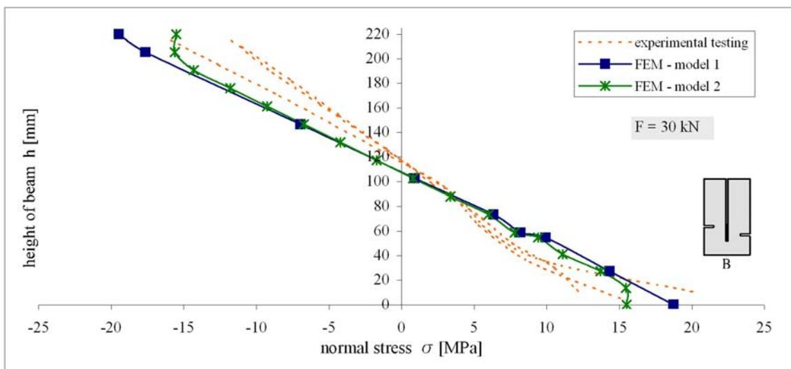
Figure 15. Graph of normal stresses in wood in beam B, force F = 30
