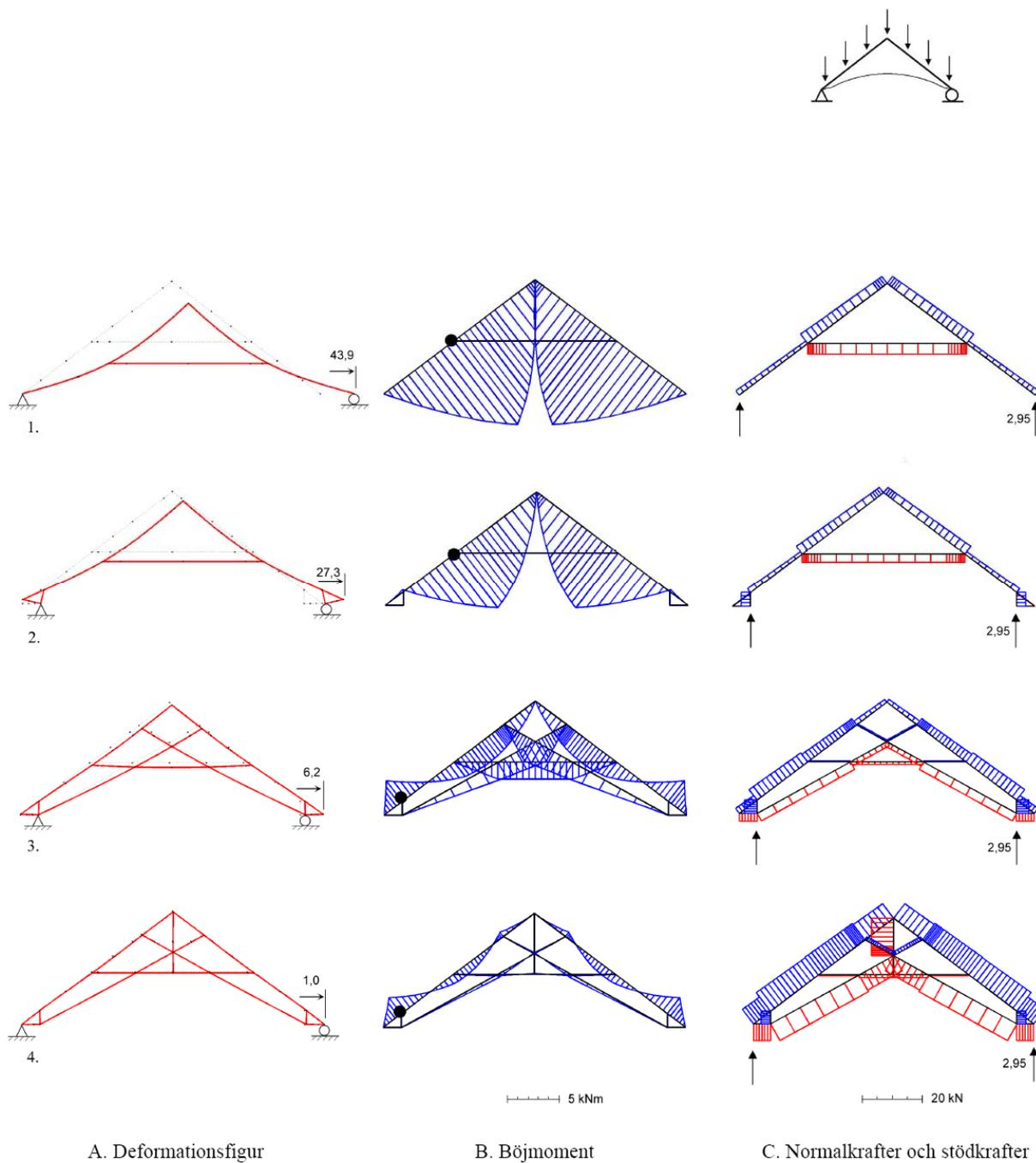
**Figure 5.** Roof trusses analysed for the 'task' type 'support by compression and tension' from Sandin [1]. To the left deflections, in the middle bending moments, and to the right normal and reaction forces
