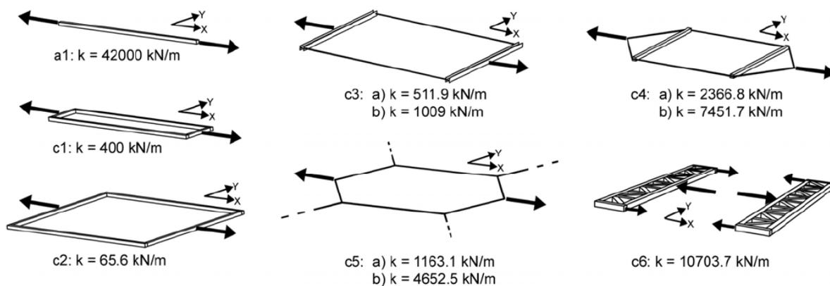
Figure 8. Stiffness that differing forms of horizontal support provide
