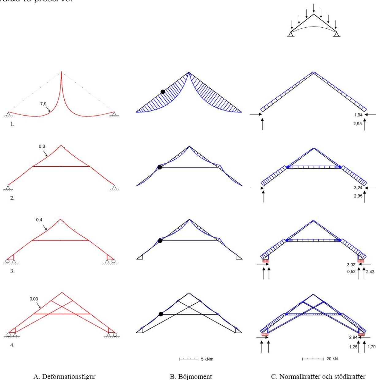
**Figure 4.** Roof trusses analysed for the 'task' type 'support as an arch' from Sandin [1]. To the left deflections, in the middle bending moments, and to the right normal and reaction forces
