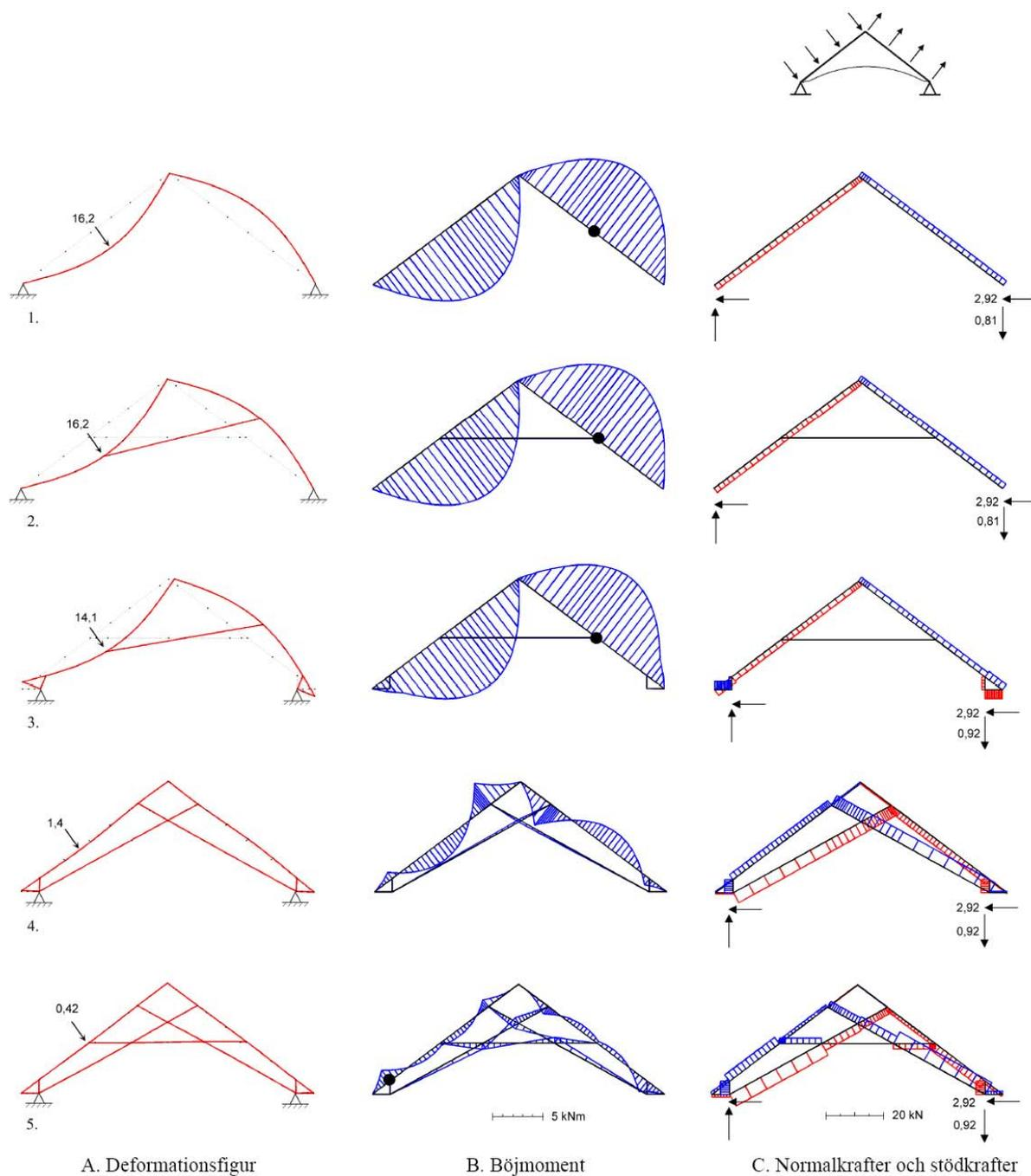
**Figure 6.** Roof trusses analysed for the 'task' type 'support as two beams' from Sandin [1]. To the left deflections, in the middle bending moments, and to the right normal and reaction forces
